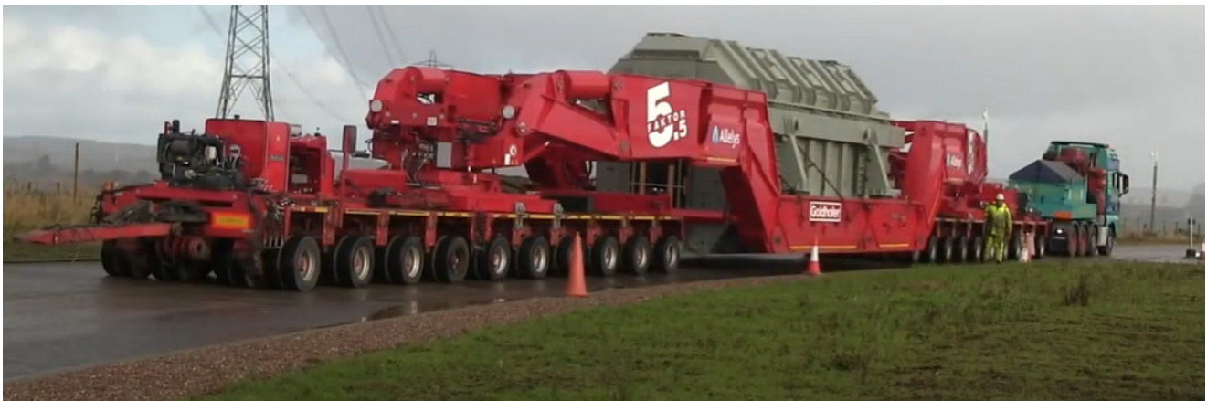
Figure 2 Example Transformer Load Transporter
